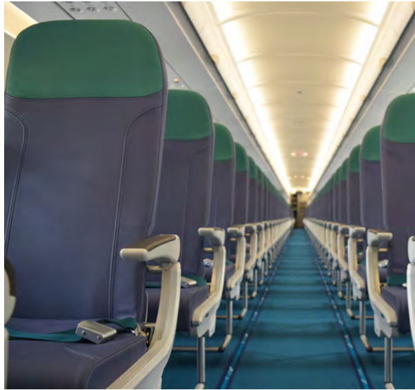
A321neo seats are made by Recaro, of lighter density material and designed with a natural incline for more comfort.
