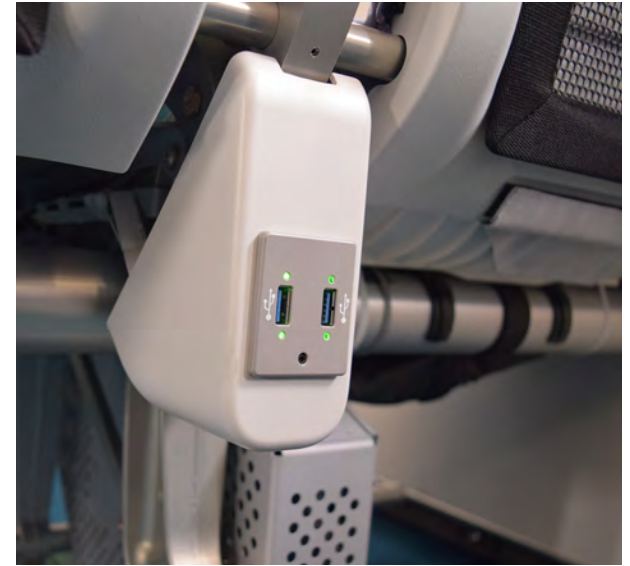
A321neo seats come with USB ports for charging of devices in-flight.
